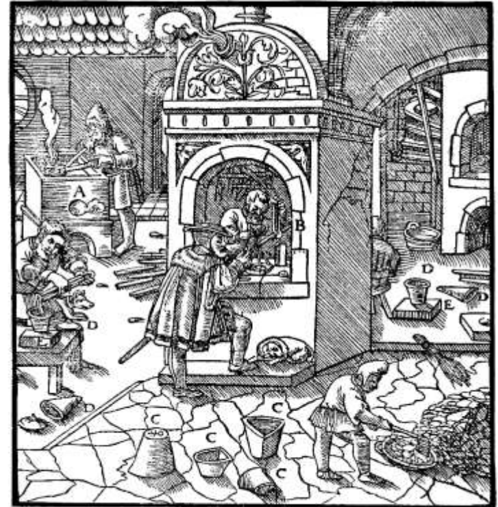
A—FURNACE IN WHICH THE AIR IS DRAWN THROUGH HOLES. B—GOLDSMITH'S FORGE. C—EARTHEN CRUCIBLES. D—IRON POTS. E—BLOCK.
