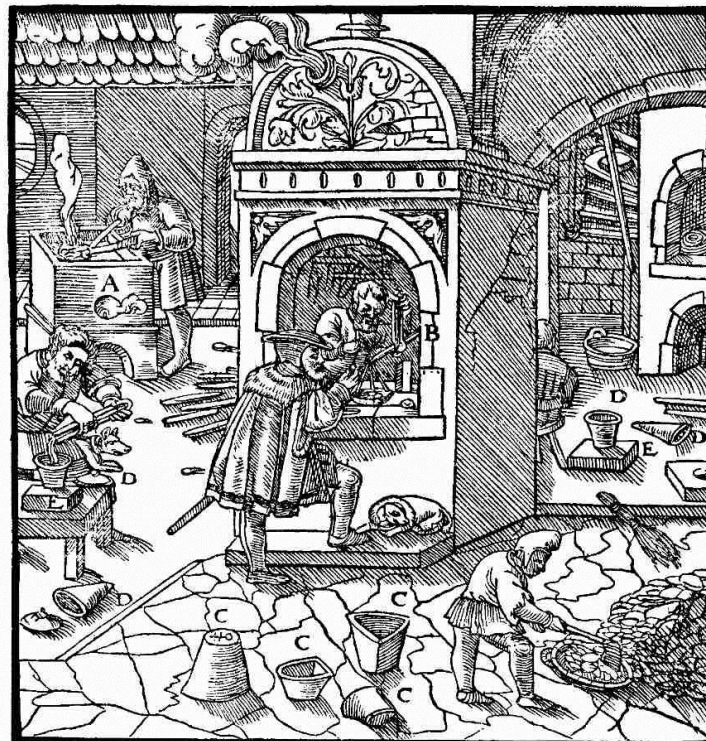
A—FURNACE IN WHICH THE AIR IS DRAWN IN THROUGH HOLES. B—GOLDSMITH'S FORGE. C—EARTHEN CRUCIBLES. D—IRON POTS. E—BLOCK.
